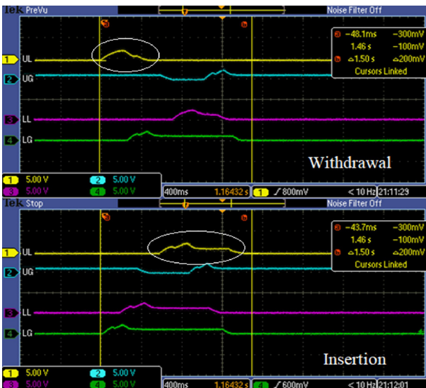
Fig. 11. Experimental results of the proposed MRAC in the abnormal condition.
