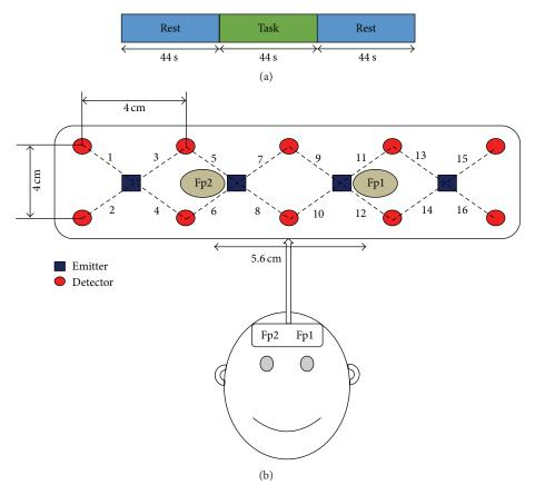
FIGURE 1: (a) Schematic of the experimental paradigm: the blue blocks represent the 44 s rest periods at the beginning and at the end; the second, green block represents the 44 s mental arithmetic task; (b) optode placement and channel location on the prefrontal cortex. Fp1 and Fp2 are the reference points of the international 10-20 system.
