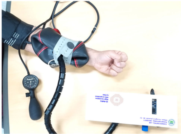
FIGURE 7. Setup for an arterial occlusion test: The cap is tied on the arm, while the gray elastic band ensures coupling of sources and the detector with the skin (the device is placed on a table).
