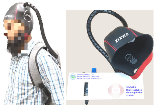
FIGURE 8. The wearable device can be placed in a backpack while the subject can wear the headgear and move freely.
