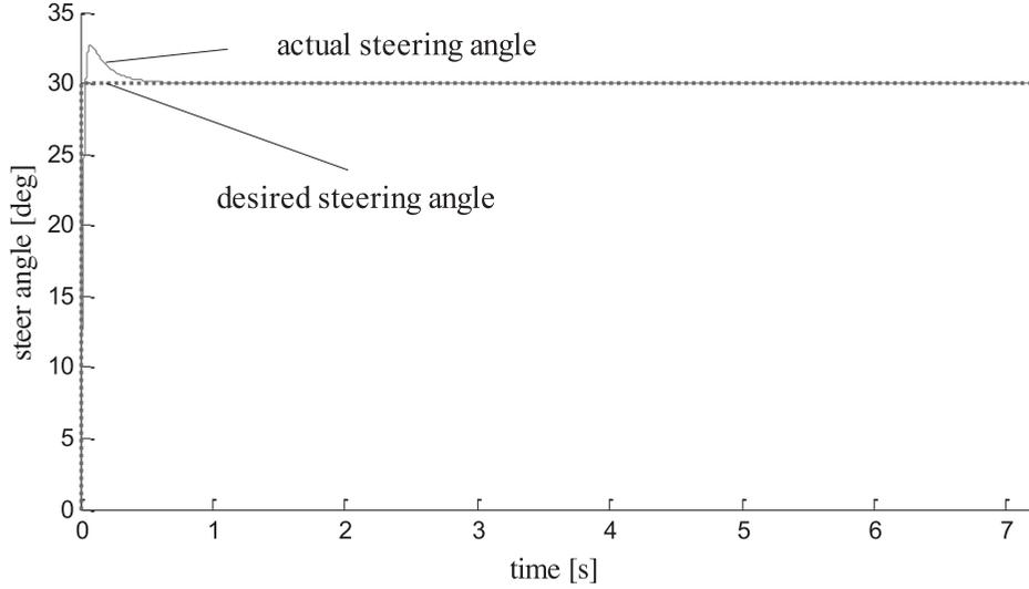
Figure 7. Steering angle profile: desired angle (dotted line,  $\omega_d = 30^\circ/\text{s}$ ) and actual angle (solid line).
