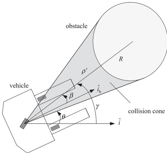
Figure 5. Collision cone.
