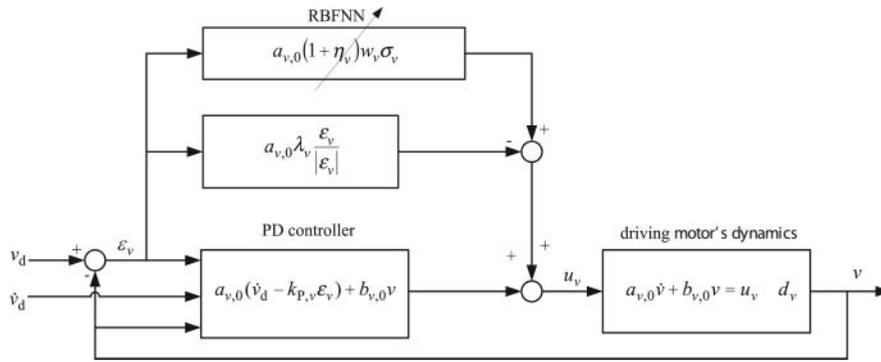
Figure 2. Control scheme of the driving motor.
