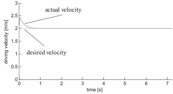
Figure 6. Driving velocity profile: desired velocity (dotted line,  $v_d = 2$  m/s) and actual velocity (solid line).
