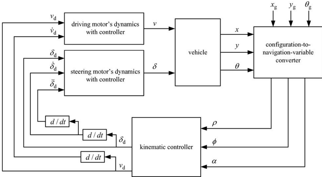
Figure 4. Motion control scheme of the vehicle.
