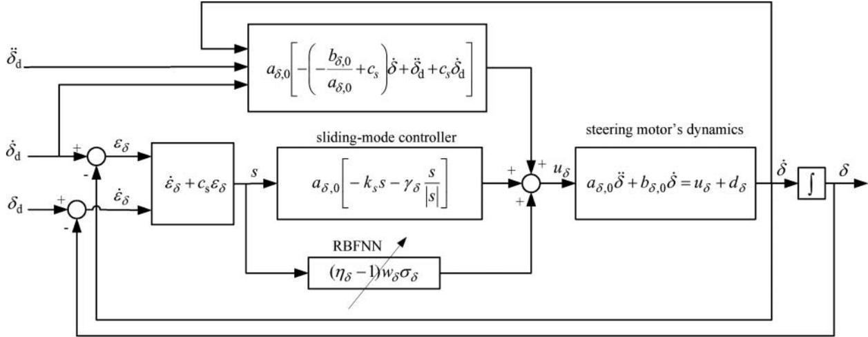
Figure 3. Control scheme of the steering motor.
