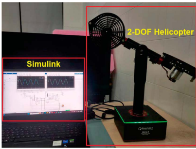
Fig. 6. Quanser Aero 2 experiment platform.
